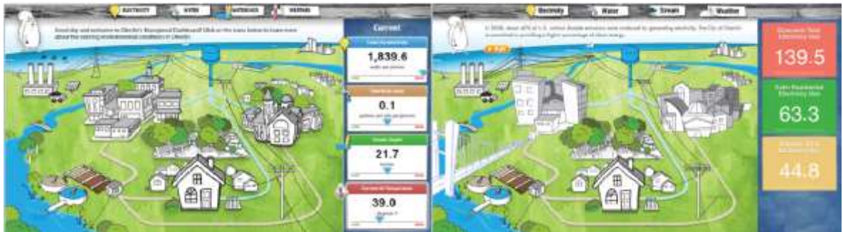
Fig. 7: Citywide Dashboard. An animated display of real-time electricity and water use and environmental conditions in entire communities or organizations. Gauges and animations of water flowing through pipes and electrons flowing down power lines reveal how decisions made in our homes and workplaces are reflected in citywide patterns and conditions. Messages delivered by “Wally Walleye” and “Flash the Energy Squirrel” narrate the story of current resource use. The goal is to situate individual decision-making in a community and systems context. The landscape has been developed with clustered buildings in order to be able to easily customize the display to feature different cities and organizations (left version features Oberlin college and city, right features Toledo and Lucas County Schools).
