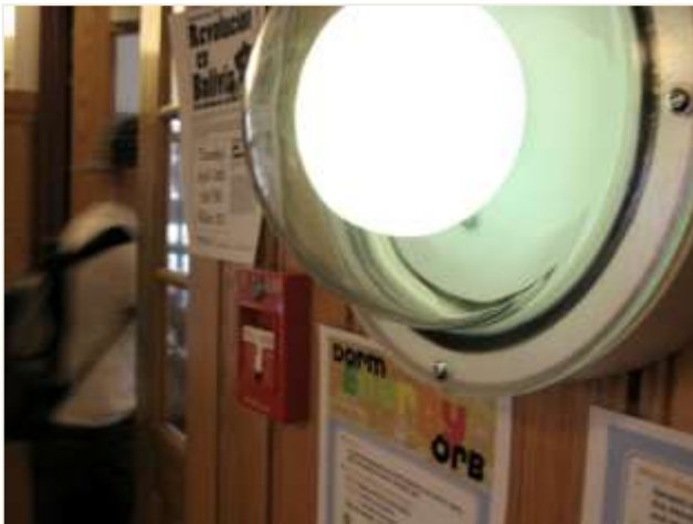
Fig. 4: “Environmental Orbs” glow different colors and with different pulsing patterns to communicate whether current levels of electricity and water consumption within a building are high or low relative to typical levels of use at this time of day. The orb pictured is installed in the lobby of a college student dormitory.
