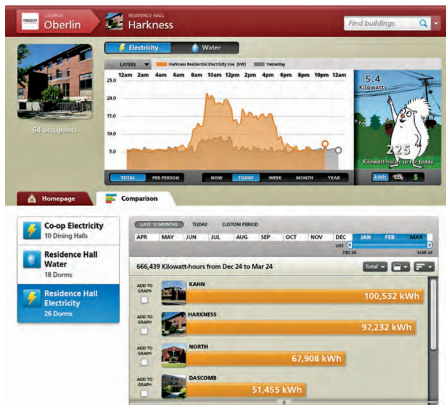
Figure 2: The Building Dashboard makes information on resource use accessible and engaging to non-technical building occupants: current patterns are compared with past performance and amongst buildings, and character gauges animate in response to resource consumption.
