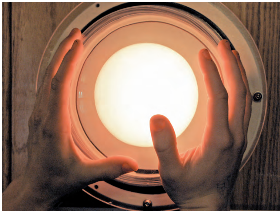
Figure 1: “Environmental Orbs” installed in the hallways of dormitories glow different colors to communicate current levels of electricity and water consumption within buildings. Our research indicates that the presence of orbs increases awareness and motivation to conserve and significantly reduces electricity consumption.
